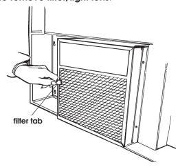
Pull firmly on filter tab to remove filter/light lens from range hood.
